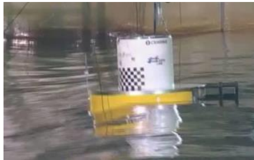
Figure 1b: Small scale wave tank model of HarshLab2 that provided training data for this study
