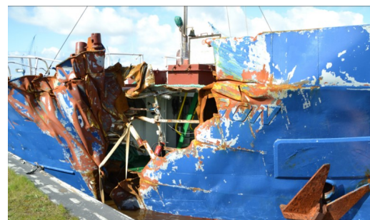
Figure 1b: The cargo ship Petra L. stroke an offshore wind turbine at GodeWind 1 wind farm (Germany). [2]
