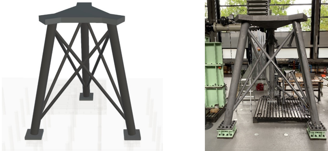
Figure 2: Design of test structure (left) / Manufactured test structure at BAM test facility with removed X joint (right).
