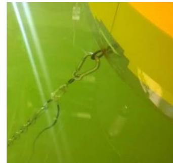
Figure 1c: Chain and load cell of HarshLab2 wave tank model's mooring system
