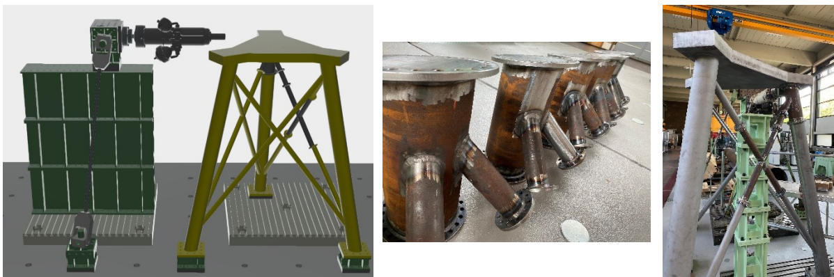
Figure 3: Facility setup for horizontal cyclic loading of test structure (left) / Removable Y joints (middle) / Manufactured test structure at BAM test facility with removable joints inserted (right).
